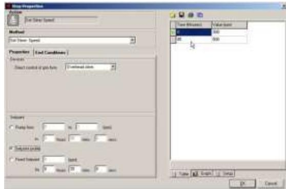
Set point profiles can be defined in two ways. They can either be added in the form of a table or graph. Selecting “set point profile” enables the profile editor.
