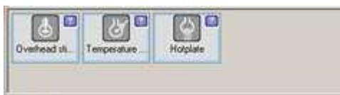
As apparatus is added it is shown with a blue question mark (as above) showing that although the apparatus is configured, Atlas doesn't have an associated recipe step for it.
