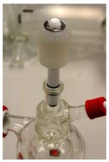
Rotate the BOV clockwise until fully closed. WARNING – Do not over tighten. Once closed, you will see a small gap between the valve handle and the circlip. **Open the valve anticlockwise by one 360° turn.** This will allow for contraction/expansion of parts and prevent damage to the vessel.
