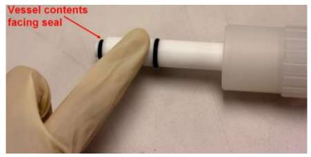
Suitable lubricants include silicone oil/grease, water or any other substance that does not effect your chemistry.
