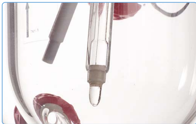
Left: pH and temperature probes in reactor
