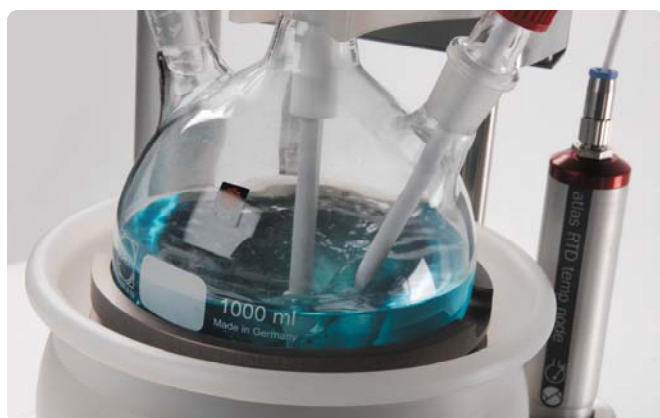
Left: A 1000ml round bottom flask heated on the Stacking Dry Bath
